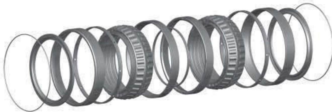
Fig. 45. sealed roll neck bearing.
