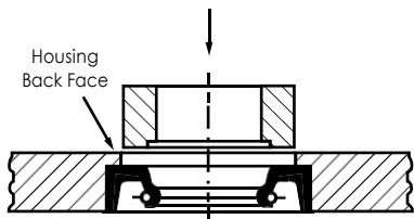
**Fig. 8. Seal removal from the back face.**
